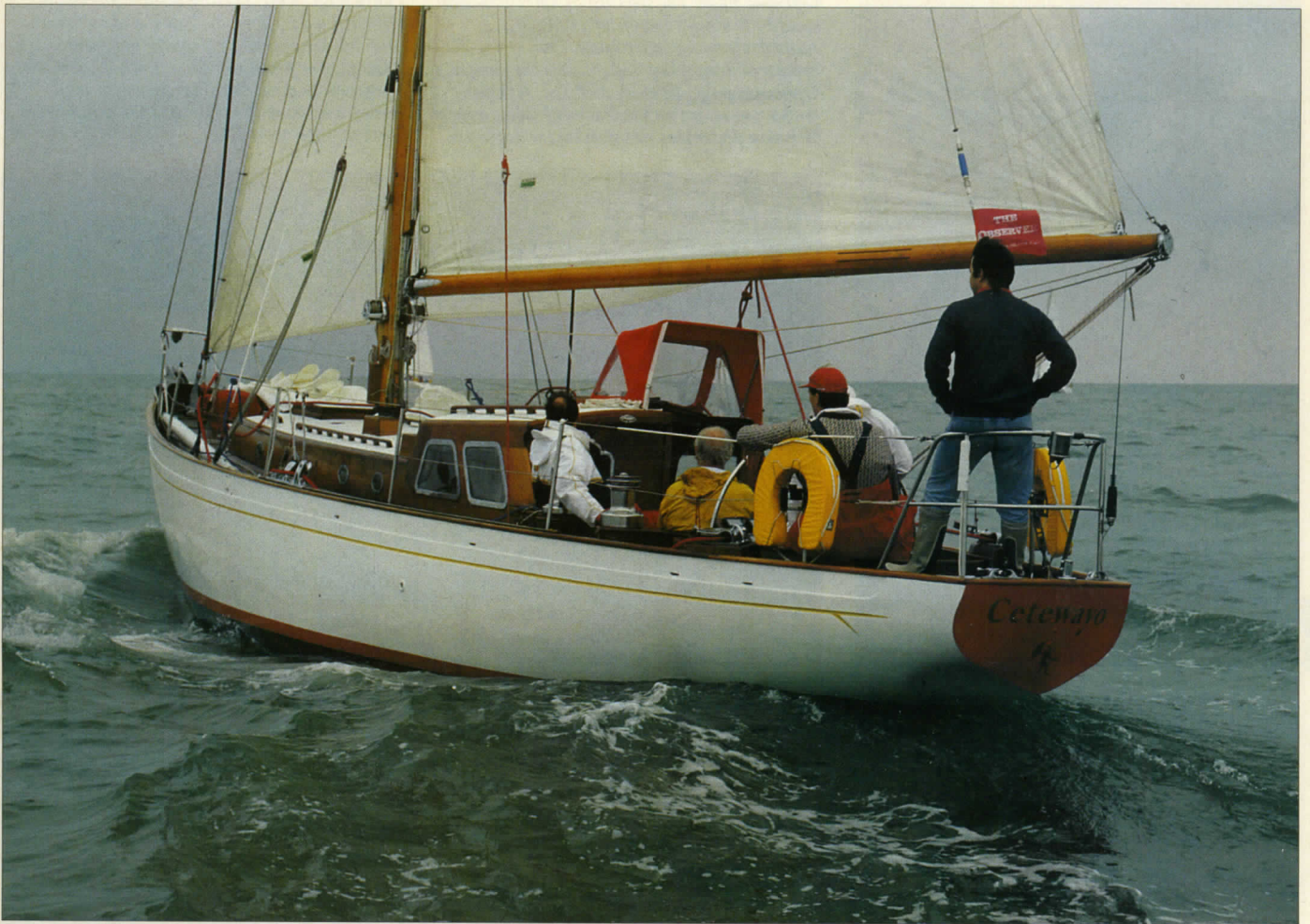
Above: Cetewayo shows the wave form typical of a deep-keeled hull, and Laurent Giles' characteristic transom. Left: The decklight is sited over the galley. Foresail lead cars run along the bulwarks. Right: Laurent Giles pattern backstay lever freed off, and large foot block under load from the foresail sheet. Below: Eat now or for ever hold your peace. Room to spare as the entire crew is seated around Cetewayo's big saloon table. Opposite page: Cetewayo's semi-circular handrail was inspired by the ex-royal yacht Bloodhound.
