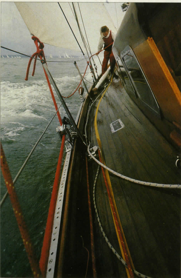
Above: Cetewayo shows the wave form typical of a deep-keeled hull, and Laurent Giles' characteristic transom. Left: The decklight is sited over the galley. Foresail lead cars run along the bulwarks. Right: Laurent Giles pattern backstay lever freed off, and large foot block under load from the foresail sheet. Below: Eat now or for ever hold your peace. Room to spare as the entire crew is seated around Cetewayo's big saloon table. Opposite page: Cetewayo's semi-circular handrail was inspired by the ex-royal yacht Bloodhound.
