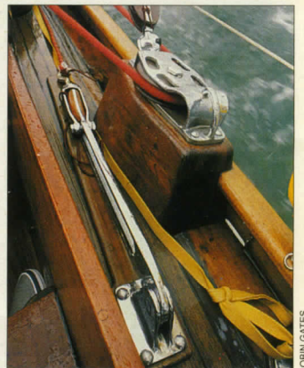
Above: Cetewayo shows the wave form typical of a deep-keeled hull, and Laurent Giles' characteristic transom. Left: The decklight is sited over the galley. Foresail lead cars run along the bulwarks. Right: Laurent Giles pattern backstay lever freed off, and large foot block under load from the foresail sheet. Below: Eat now or for ever hold your peace. Room to spare as the entire crew is seated around Cetewayo's big saloon table. Opposite page: Cetewayo's semi-circular handrail was inspired by the ex-royal yacht Bloodhound.
